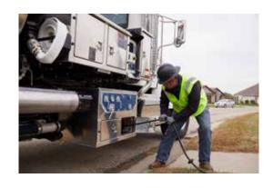
All water valves are located in the same mid-ship control station, reducing the amount of walking back and forth around the truck by the operator
