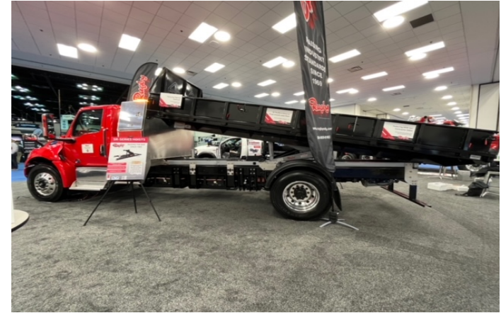
Rugby's Vari-Class body platform on a fully electric class 7 chassis
