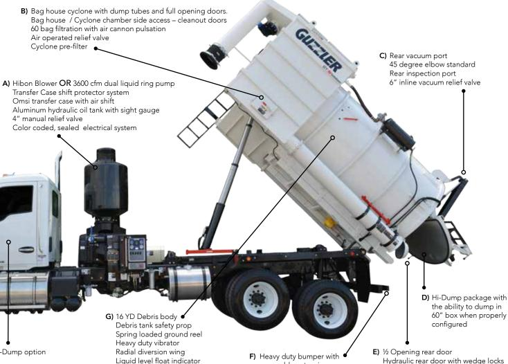
H) Custom chassis with Hi-Dump option Fire extinguisher 5 lb Guzzler manual and CD version Inclinometer and Hi-Dump control in cab Liquid level float indicator Back up Alarm Liquid level ball shut off
