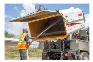
The smooth hopper design and 50-degree dump angle could make Elgin Sweeper's RegenX the easiest sweeper to clean in the industry.
