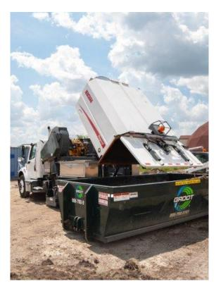
The RegenX is the only sweeper in the industry to offer the ability to dump into roll-off containers while still boasting an impressive 8yd3 capacity.
