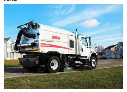
Elgin Sweeper today introduced an innovative single-engine configuration of its popular Crosswind® regenerative air sweeper. A variable-speed device installed between the chassis engine and transmission on the new configuration allows the engine to simultaneously power both the truck and the sweeper.
